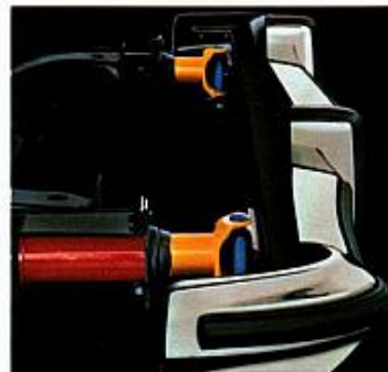
Left: Energy absorber-type mounts on new improved front bumper; Below: Standard Luxury LeMans fender skirt; Bottom: Luxury LeMans scroll on front armrest; Right: Standard notchback bench seat in cloth and vinyl.
