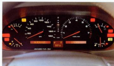
The Driver Information System insulates and prioritizes 22 functions; a flip of the column stalk activates a convenient 10-function onboard computer.
